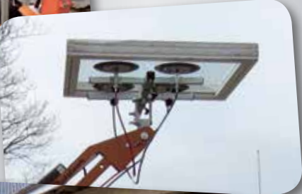
The Smartlift can be shifted sideways for precision adjustment during installation jobs.
